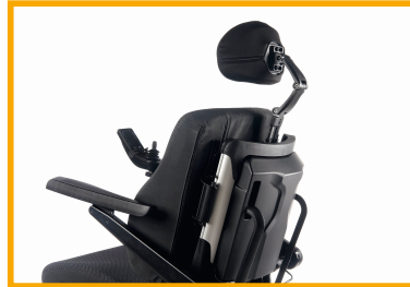
User Adjustable Manual Recline Back, 90°-130° Shifting body weight made easy with gas spring. Operating lever for user adjustment under the armrest.
